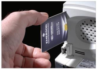
Emerson's SmartCard is a memory device that ships with every Unidrive SP, Mentor MP, Quantum MP and Digitax ST Control Techniques' motor drive. The card enables simple configuration of parameters in a variety of ways. Primarily, the card is used to back up parameter sets and PLC programs from one drive and copy them to another effectively "cloning" the drive.
