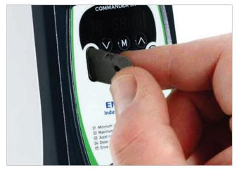
The SmartStick memory device can be used to upload drive parameters for storage or for easy set-up of identical Commander SK drives. The SmartStick cloning module provides fast and cost-effective drive-to-drive parameter transfer and storage without a PC. A drive can be set to boot from the SmartStick on every power cycle.
